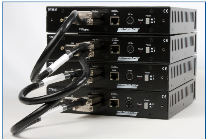
Figure 2. Up to sixteen modules may be used in parallel to connect a possible 64 direct voltage or IEPE channels, each synchronized in a master/slave configuration. The picture above shows four instrument modules in such a configuration.
